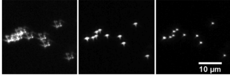
Figure 4: Comparison of images of 200 nm diameter fluorescent beads: left image without correction showing the deformable mirror induced aberrations; center image showing residual setup aberrations; right image showing nearly perfect aberration correction.
