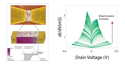
The migration of oxygen vacancies by an electric field has been employed recently for the fabrication of memristive devices, devices that could possibly become essential in future Von Neumann or neuromorphic computing architectures. In these devices, the oxygen vacancies play the role of doping sites.
